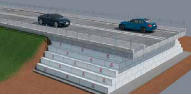
Figure 1 Usage that lighten the design load instead of the earth fill used in highways, bridges and approaching ramps.
