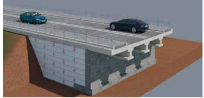
Figure 2 Prevention of settlement in bridge approach constructions and slope filling on soft soil surface.
